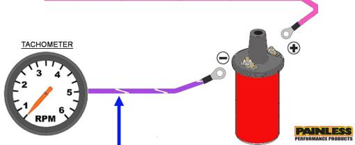
[ENGINE SECTION] <<COIL(-) #923 TACHOMETER SIGNAL >>[INSTRUMENT PANEL]
